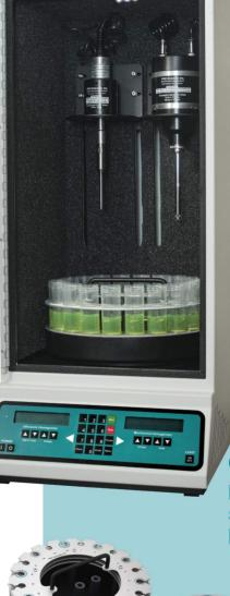
Cooling Carousel Racks protect and keep your samples cool during homogenization.
